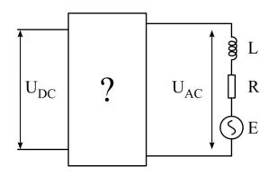
Inverters are devices that convert **DC** voltages/currents into **AC** voltages/currents.
