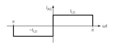
$$A_{h} = \frac{1}{\pi} \int_{-\pi}^{\pi} i_{AC}(\omega t) \cdot \cos(h\omega t) \cdot d(\omega t) \qquad A_{h} = 0$$
