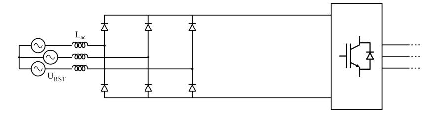
Additional circuitry that secures proper rectifiers operation:
