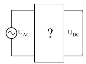
Rectifiers are devices that convert **AC** voltages/currents into **DC** voltages/currents.
