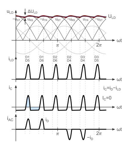
Three-phase diode (uncontrolled) rectifier
